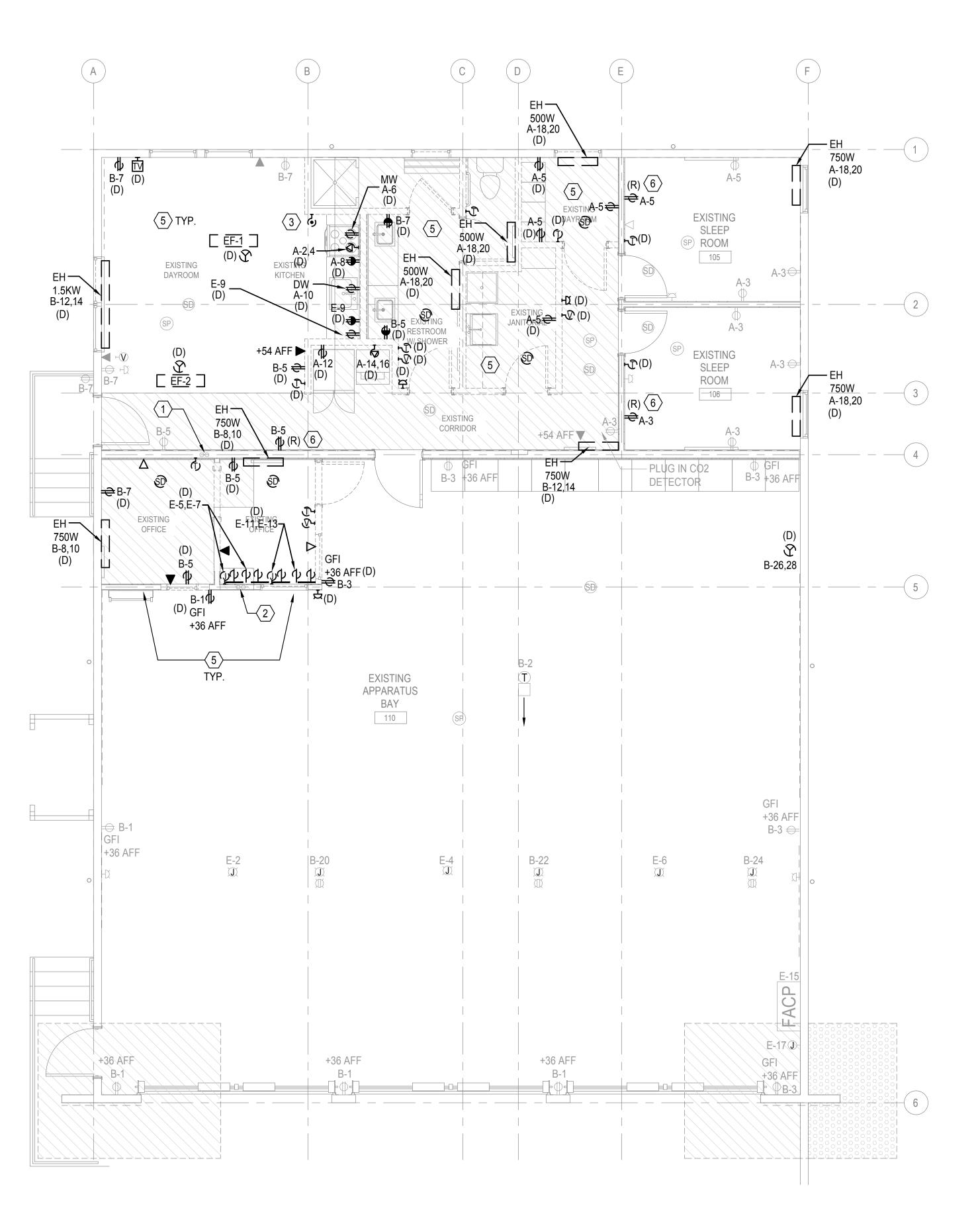
N DEMOLITION FLOOR PLAN - LEVEL 1 - POWER SCALE: 1/4"=1'-0" FLAG NOTES X:
